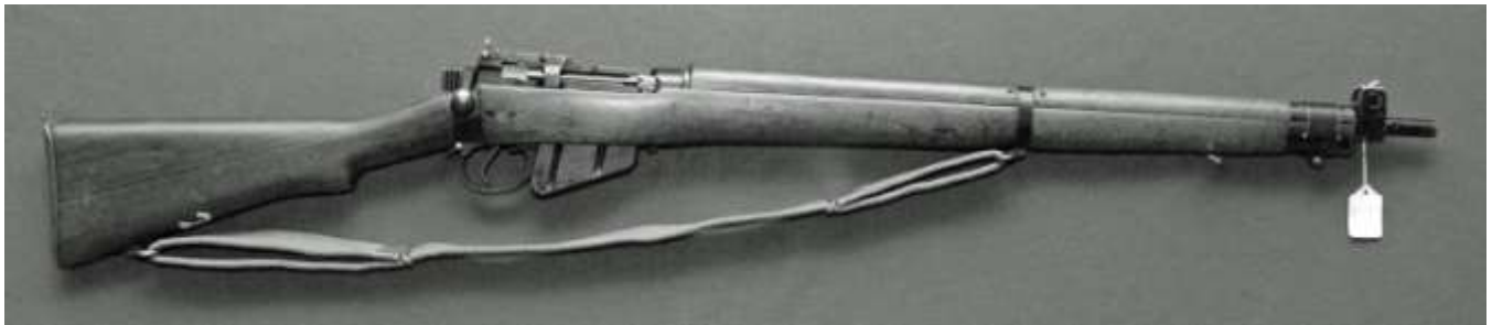
Lee-Enfield No4 Mk1 (WWII and on) – note receiver (peep) sight and protruding muzzle. “Spike” Bayonet.
