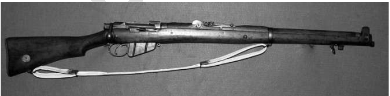
* Short, Magazine Lee-Enfield Mk I *** - short rifle with sliding charger guide mounted on bolt head. P1903 / P1907 Bayonet
